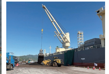
Unloading of bulk cargo
